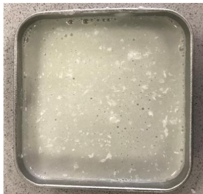
Figure 7. Undissolved particles observed during outer layers development using solvent evaporation method.
