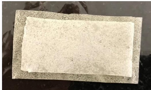
Figure 5. Developed triple layered system with the outer layers covering the internal layer.
