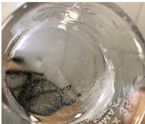
Figure 10. Slightly viscous solution obtained during internal layer development using solvent evaporation method.
