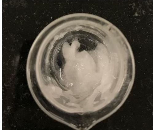
Figure 8. Gel formation during outer layers development using solvent evaporation method.
